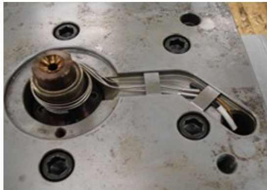
Figure 6-63: Wire Wrapped Around Sprue Heater (Example)
