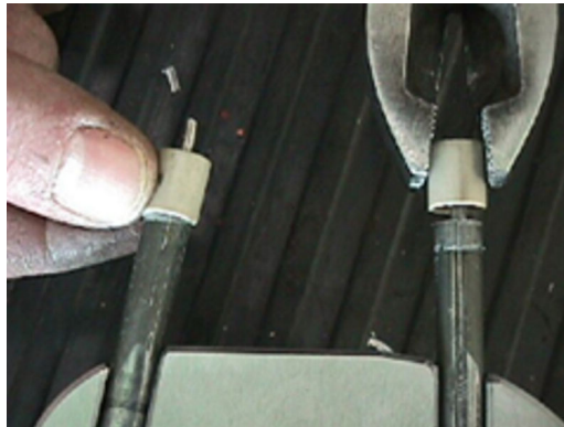
Figure 6-65: PEEK Bushing Removal and Installation
